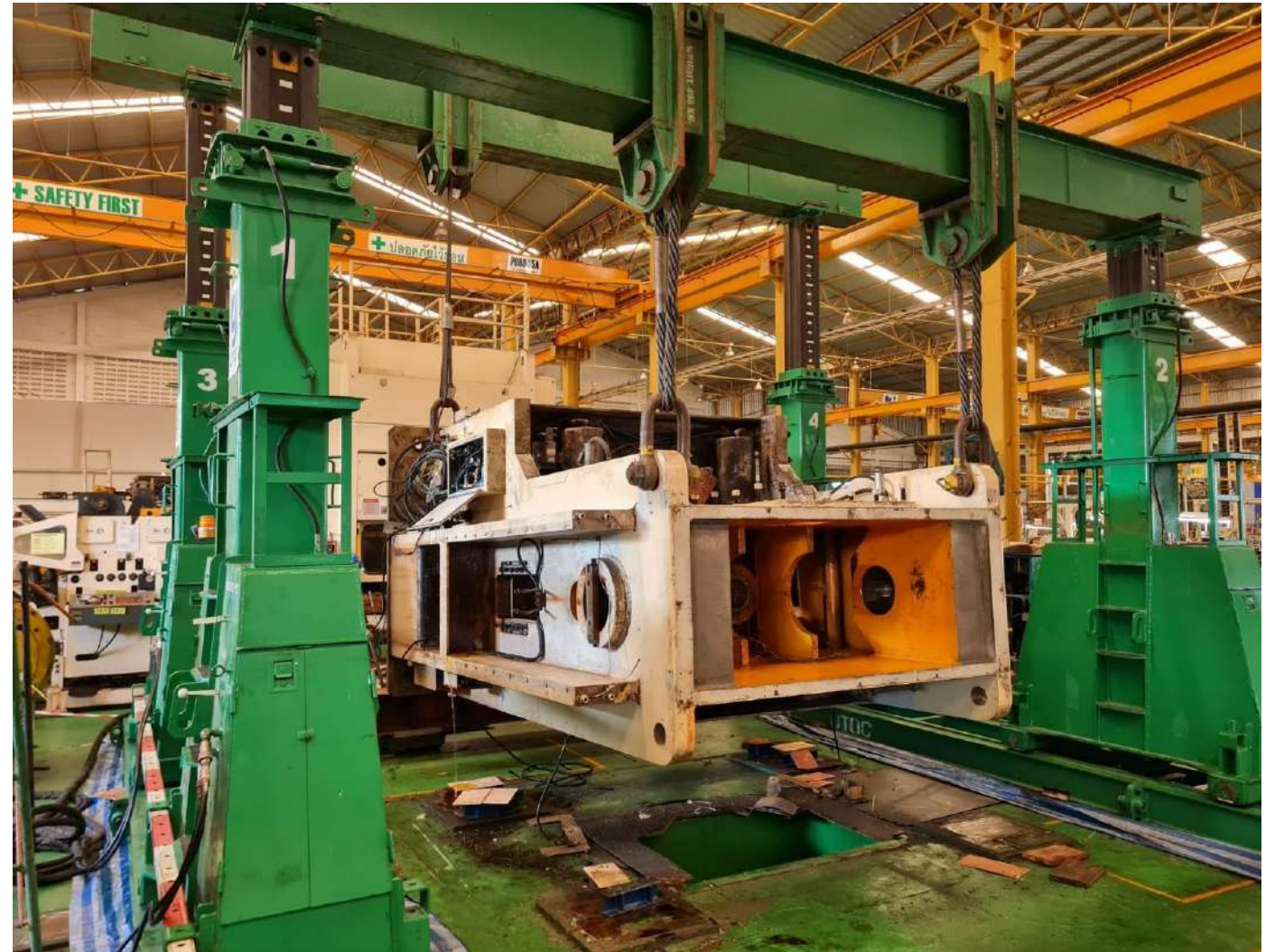
Disassembly 600 Ton Patec Press (Bolster 2100 x 1000 mm) . Machine Weight: 68 ton
