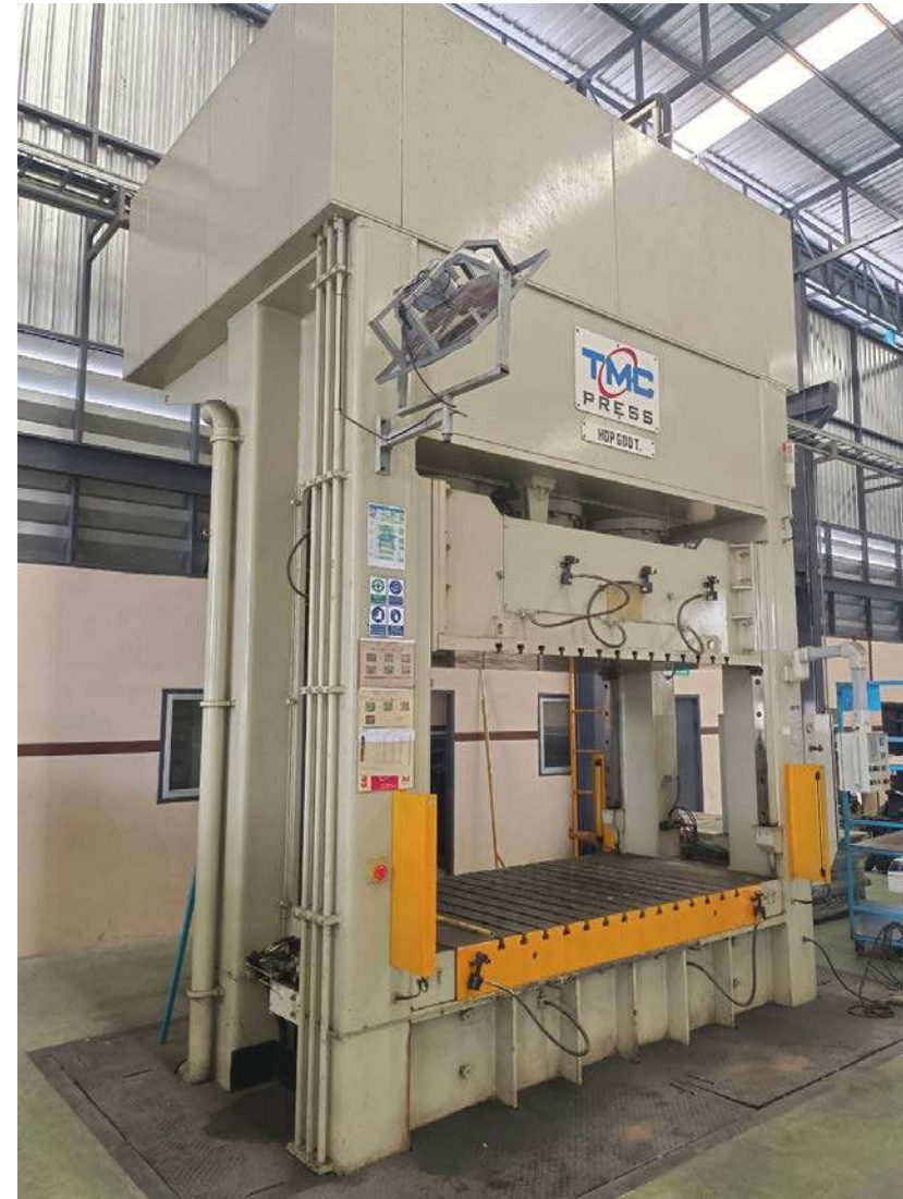
Installation of TMC 600 Ton Hyd. Press. Machine Weight: 55 ton
