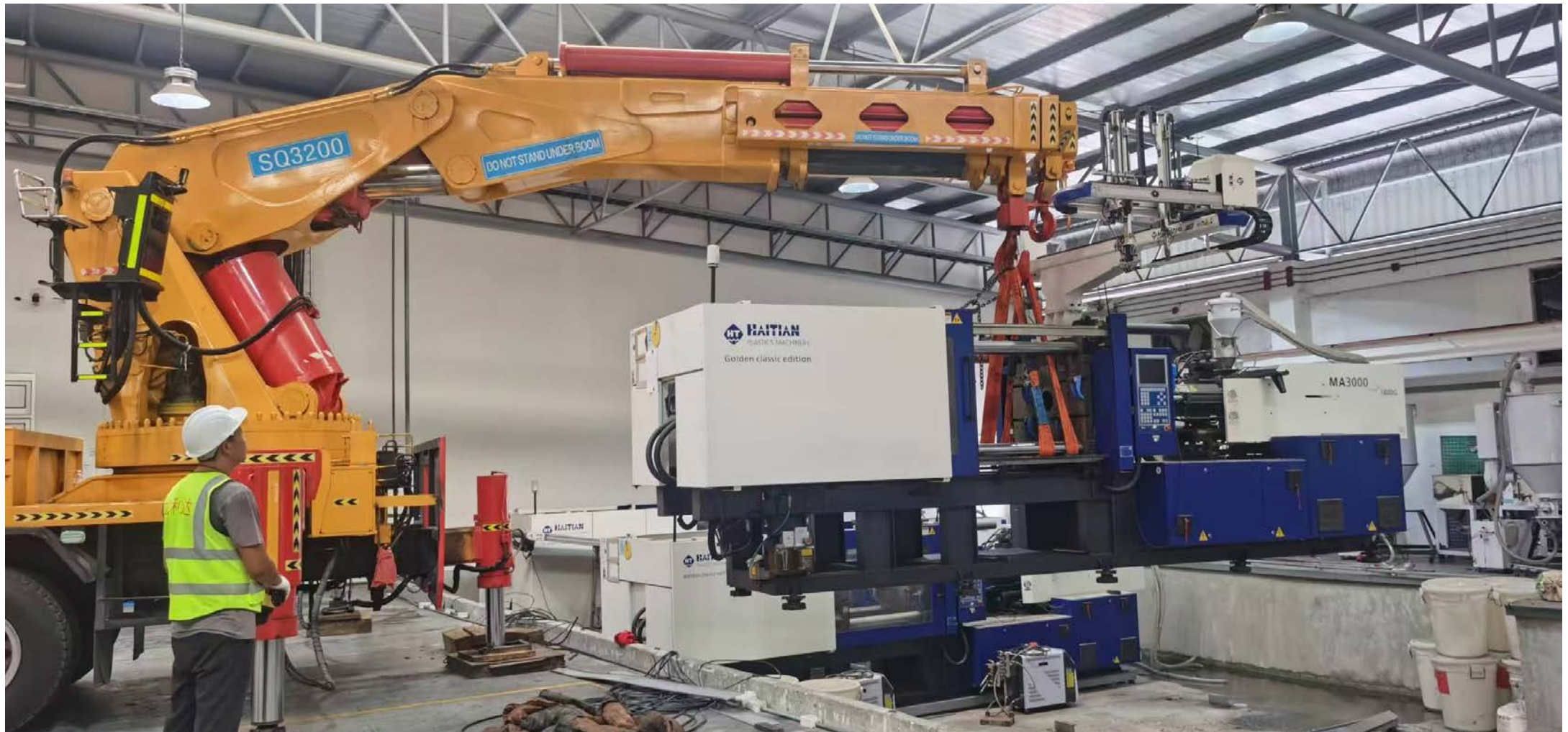
300 Ton Haitian Injection Machine. Weight: 12 ton
