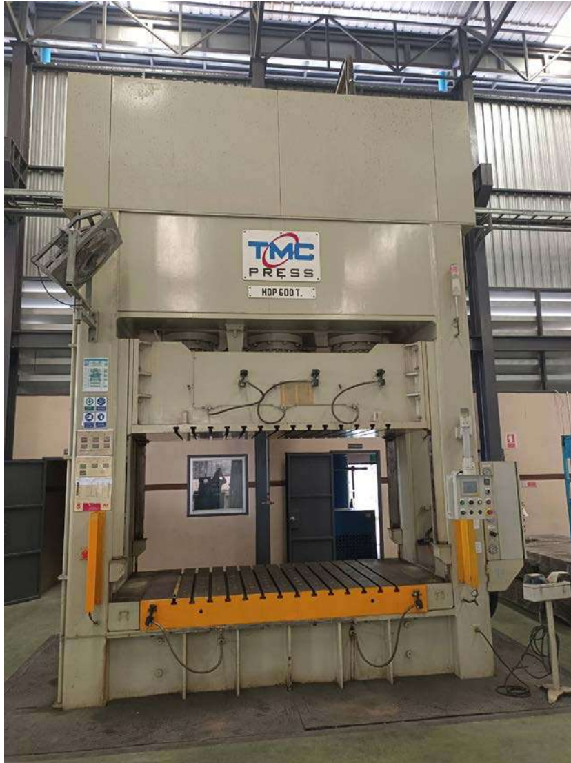
Installation of TMC 600 Ton Hyd. Press. Machine Weight: 55 ton
