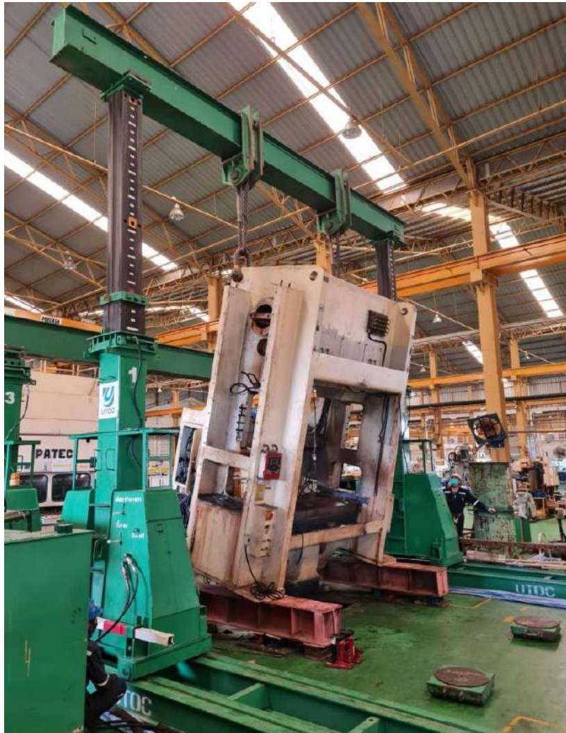
Disassembly 600 Ton Patec Press (Bolster 2100 x 1000 mm) . Machine Weight: 68 ton
